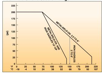
These ratings are for PVC and PVDF fittings. For all metal fittings 10" and larger, a PVC insert is used; for 8" and below, a PVDF insert is used. Use the appropriate curve to determine the maximum pressure rating of these fittings.
