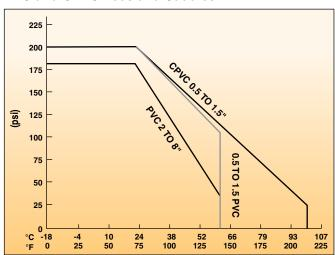
WARNING: THE ABOVE PRESSURE/TEMPERATURE CURVES ARE SPECIFICALLY FOR THE FPL300. FPL3001, AND FPL3003 SENSORS. DURING SYSTEM DESIGN, THE SPECIFICATIONS OF ALL COMPONENTS MUST BE CONSIDERED. IN A METAL PIPING SYSTEM, A PLASTIC SENSOR WILL REDUCE THE SYSTEM SPEC. ON THE OTHER HAND, IF USING A PVDF SENSOR IN A PVC PIPING SYSTEM, THE FITTING WILL REDUCE THE SYSTEM SPEC.
