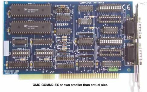
is also capable of RS232 for applications requiring shorter distances and RS232 compatibility. Signals are transmitted and received via two 9-pin sub-D connectors. Bit character lengths of 5, 6, 7 or 8, and odd, even or no parity are all available.
