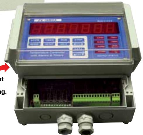
CN1511 has removable front cover for easy access to wiring.
